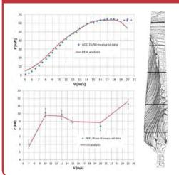
Validation of steady / unsteady RANS CFD models and BEM model using data of SANDIA and NREL turbines:
