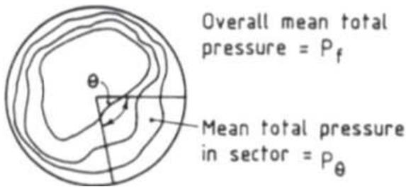
**Figure 1: Illustration of total-pressure contours and  $\theta=60$ deg sector for definition of distortion coefficient [7].**
