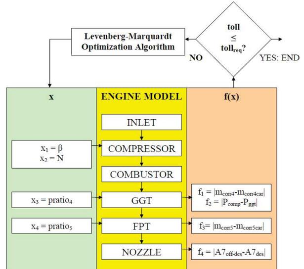
Figure 4: Matrix method used by the Off Design solver for the turboshaft engine of Figure 3.
