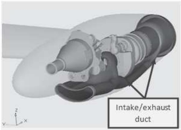
**Figure 11: Layout of the ERICA nacelle internal components. Courtesy of GRC2 Consortium.**
