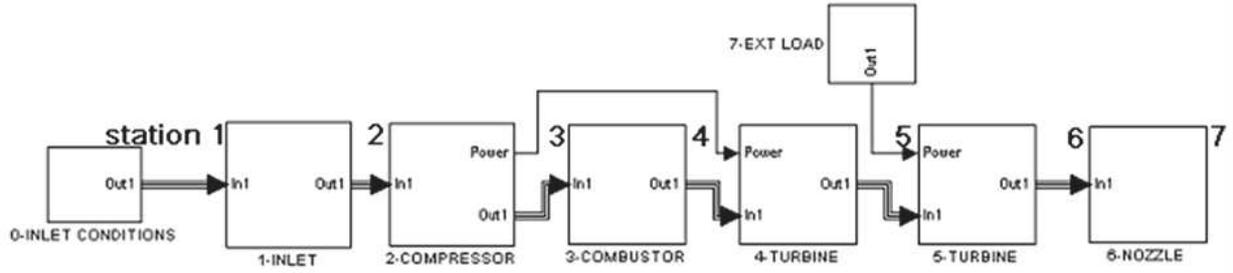
Figure 3: GE T700 engine simplified model implemented in gas turbine simulation code TSHAFT.
