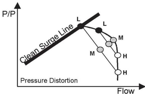
**Figure 2: IFD operating points on the same corrected speed line: L represents the distorted sector, H the clean sector and M is the average operating point (courtesy of Kurzke [8]).**
