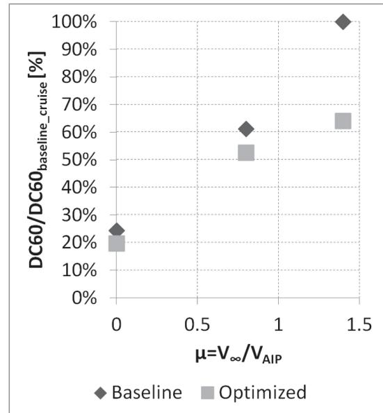
Figure 17: DC60 comparison between the baseline and optimized intake, considering cruise, conversion and hover flight conditions.
