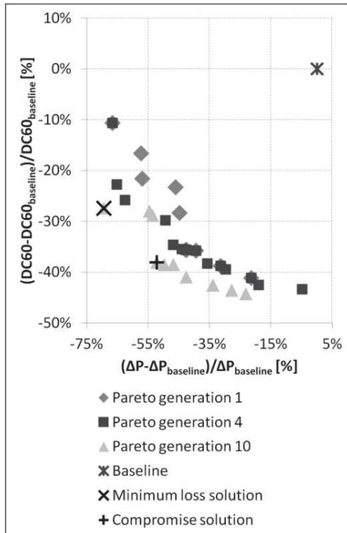
Figure 15: Intake Pareto front after 10 GDEA generations. Evolution through generations and baseline values are also represented [6].
