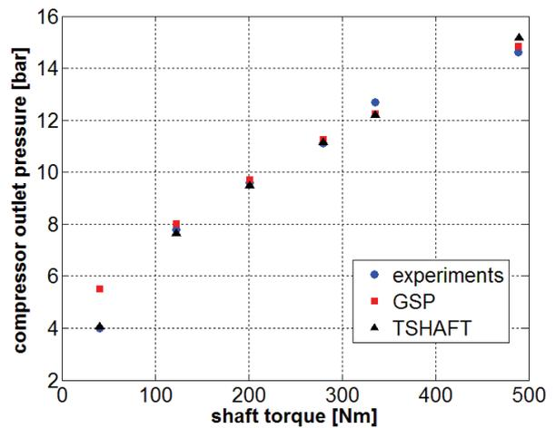
Figure 10: Compressor outlet pressure.
