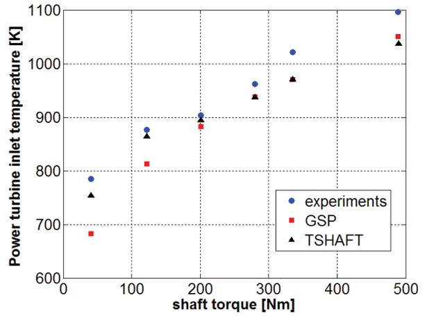
Figure 8: Power turbine inlet temperature.
