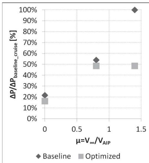
Figure 16: Total pressure loss comparison between the baseline and optimized intake, considering cruise, conversion and hover flight conditions.
