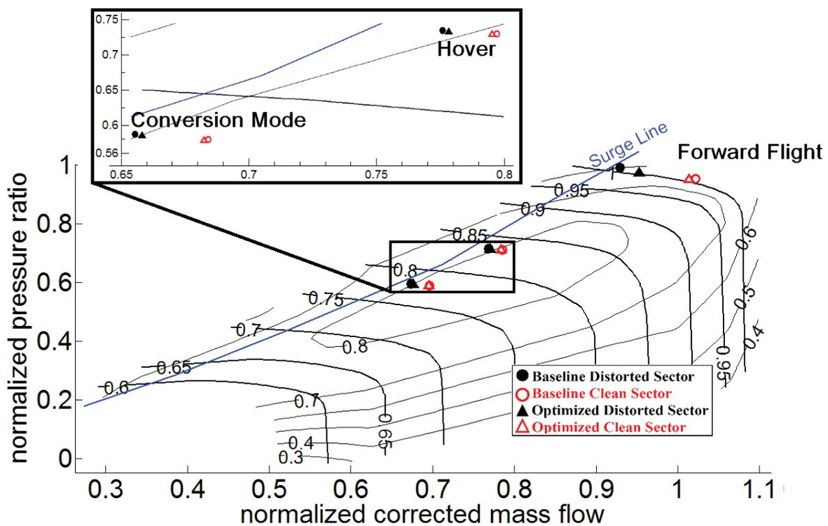
Figure 13: LP Compressor characteristic map with operating points for the three cases considered, calculated with the Parallel Compressor Model: comparison between baseline and optimized intake geometries. Normalization is carried out with respect to the cruise condition.
