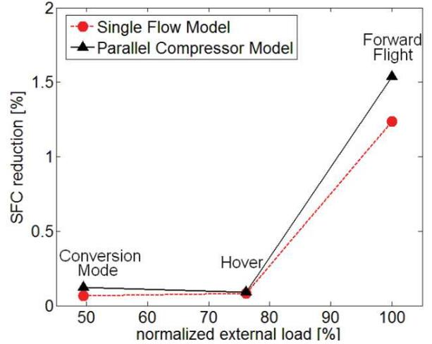
**Figure 12: Percentage SFC reduction vs. normalized external load calculated with the Single Flow Model and the Parallel Compressor Model.**
